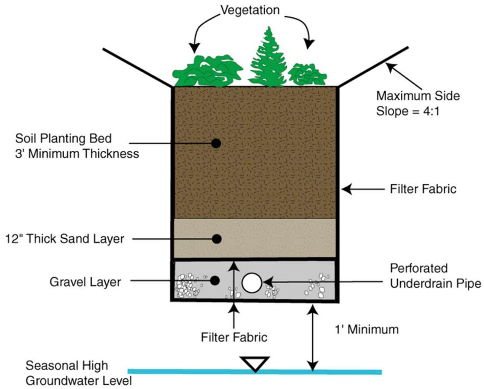
**Typical Bioretention Section Detail**
