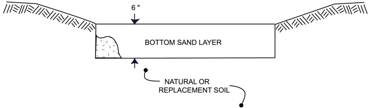
**Typical Infiltration Section Detail**
